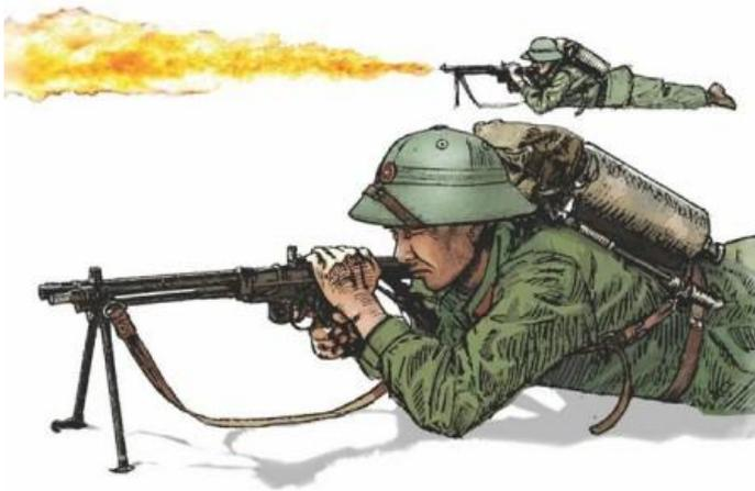
The Type 74 was a license-built copy of the Soviet LPO-50 that entered service in 1953. It had three tanks, each containing a pressure cartridge and about a gallon of special diesel fuel. The tanks were topped by a pressure relief valve and a filling
