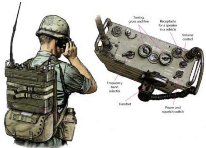
The radio had two antennas, a 3-foot standard antenna for most missions and a 10-foot long-range antenna carried in a canvas bag attached to the radio’s side. U.S. Special Forces and long-range reconnaissance patrols developed improvised “jungle antennas” that extended the range even farther.
