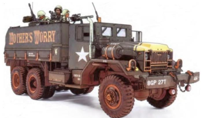
The M54 5-ton gun truck was the most common transport vehicle converted. The first conversions used a truck-bed mounted compartment for two machine guns. The crews usually placed an M60 7.62 mm forward and an M2 .50-caliber in the
